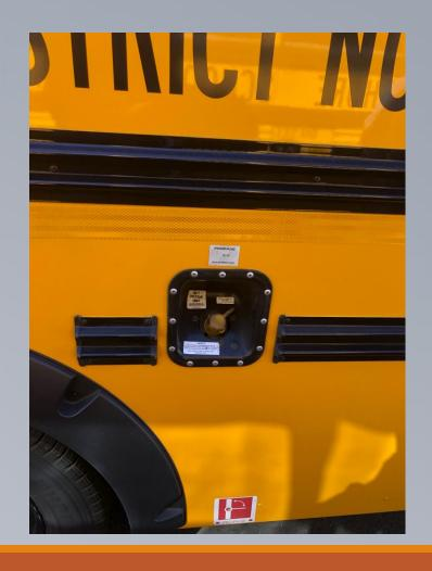
Fill location for LPG. These buses in the NSD are the 'short' busses, no current full size LPG busses.
